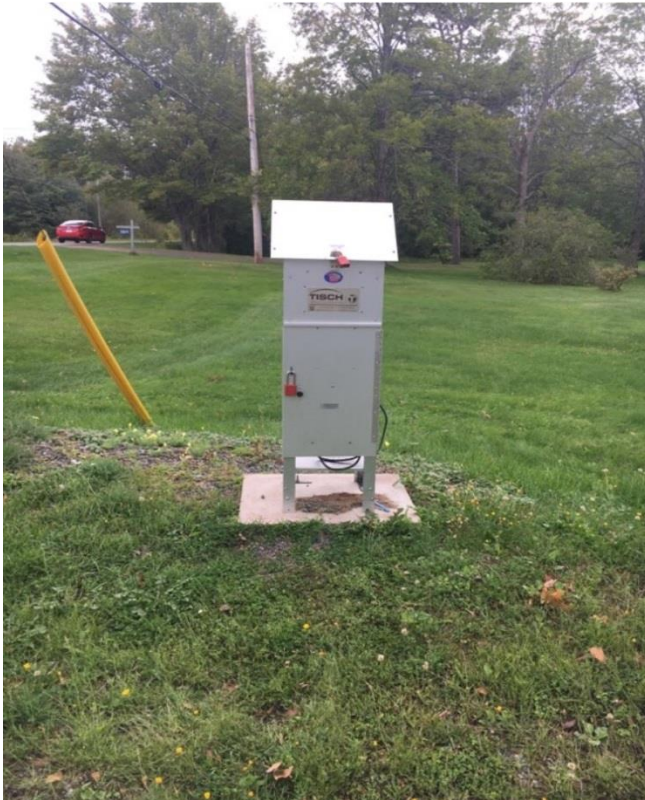
Figure 3 : Tisch Hi-Vol Total Particulate Sampler at Pictou Landing
